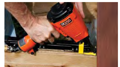
Gunnable Installation Option Installs Standard or End Seam Fastener
